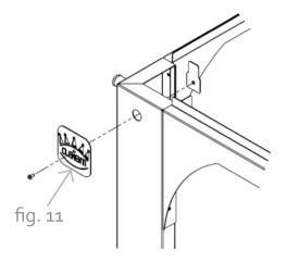
**Step 7)** The final step is to screw fig. 11 to the front left of the stand.
