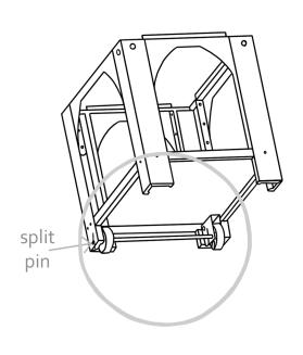
**Step 6)** Slide fig. 9(x2) into the holes on the left side of the stand as seen in the image to the right.
