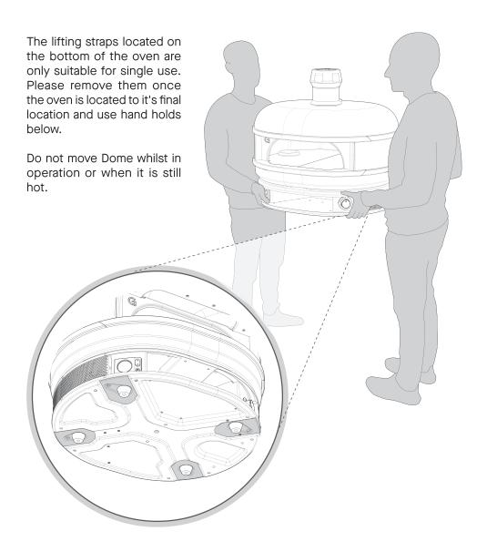
Never attempt to move the oven on your own. Two people should pick up the oven lifting from under the rounded ends of the oven, do not use the mouth of the oven as a lifting point.
