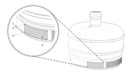
Double check the probe is functioning by checking the digital temperature display and return the panel to the back of the oven.
