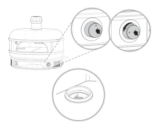
To ignite the pilot light press the control knob in until you hear a constant clicking sound. Then, still pressing, turn the knob 90° and hold it there until the pilot light is lit. You may not be able to see the naked flame but there should be clear reflections of it on the internal sides of the oven.
