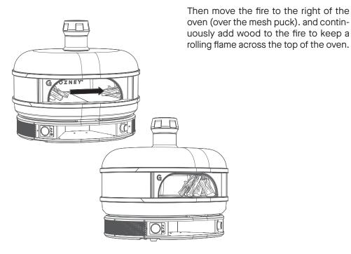
The flame from the wood fire should roll across the length of the oven's roof. Avoid overfeeding the fire, there should never be flames coming out the mouth of the oven. If you are struggling to get a good flame, ensure the wood you are using follows our guidelines at the beginning of this chapter.
