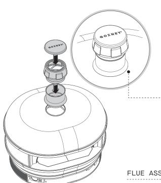
The flue is designed to have a rain guard which has a 5mm gap from the Dome.
