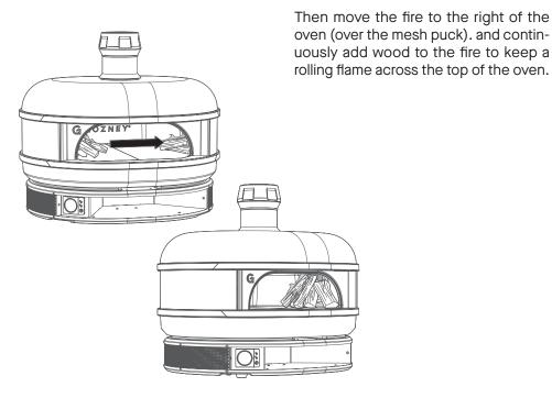
The flame from the wood fire should role across the length of the oven's roof. Avoid overfeeding the fire, there should never be flames coming out the mouth of the oven. If you are struggling to get a good flame ensure the wood you are using follows our guidelines at the beginning of this chapter.
