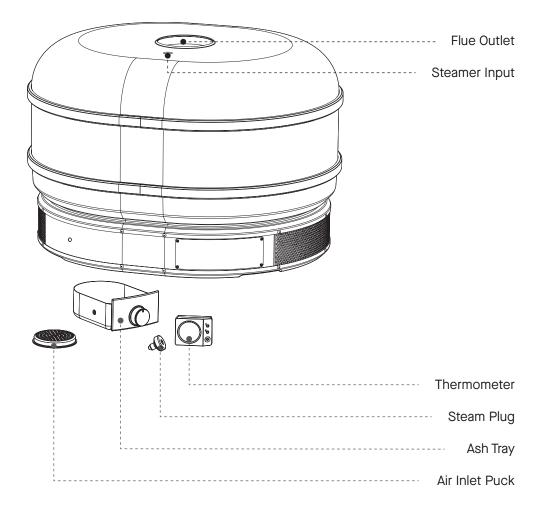
This section details the correct operation and install of a Gozney Dome.
