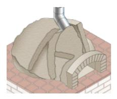
Once you have loosely laid the insulation around the oven, it is time to attach chicken wire to the hooks that you earlier drilled into the base structure. Pull the chicken wire around the oven encasing the insulation layer and form your shape. You can pack additional fireproof insulation in if your shape is not even. Once a satisfactory shape and finish is achieved, tie your chicken wire to the hooks using metal wire or cable ties to secure it in place.
