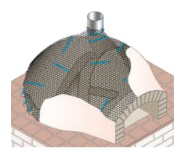
With a trowel apply this to the mesh ensuring an even coat of render is applied to the entire external surface of the oven, until the entire oven is covered. Wait for the render to be 90% set and then wipe it over with a damp sponge, to work out any trowel lines and to create a smooth surface.
