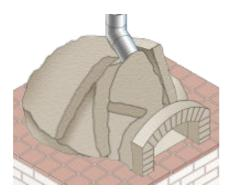
Once you have loosely laid the insulation around the oven, it is time to attach chicken wire to the hooks that you earlier drilled into the base structure. Pull the chicken wire around the oven encasing the insulation layer and form your shape. You can pack additional fireproof insulation in if your shape is not even. Once a satisfactory shape and finish is achieved, tie your chicken wire to the hooks using metal wire or cable ties to secure it in place.
